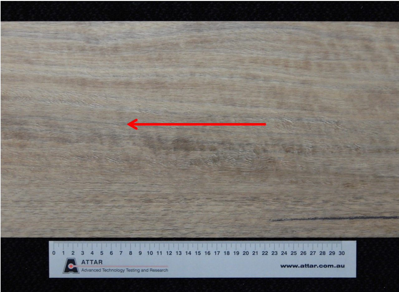
Figure 1: Kenbrock Duraplank XL Arrow indicates direction of testing
